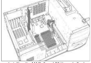
Installing the MACh Speed G3 Upgrade Card
